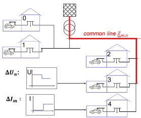
For each start of a charging cycle (Switch Event) on bus m we notice a voltage drop on bus n and derive the common line impedances:
