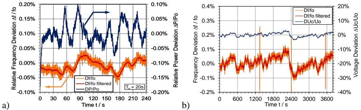
Figure 2: Measured frequency and calculated values on a capacitor with 300 Ws. a) Additional power flow. b) Voltage fluctuation,
