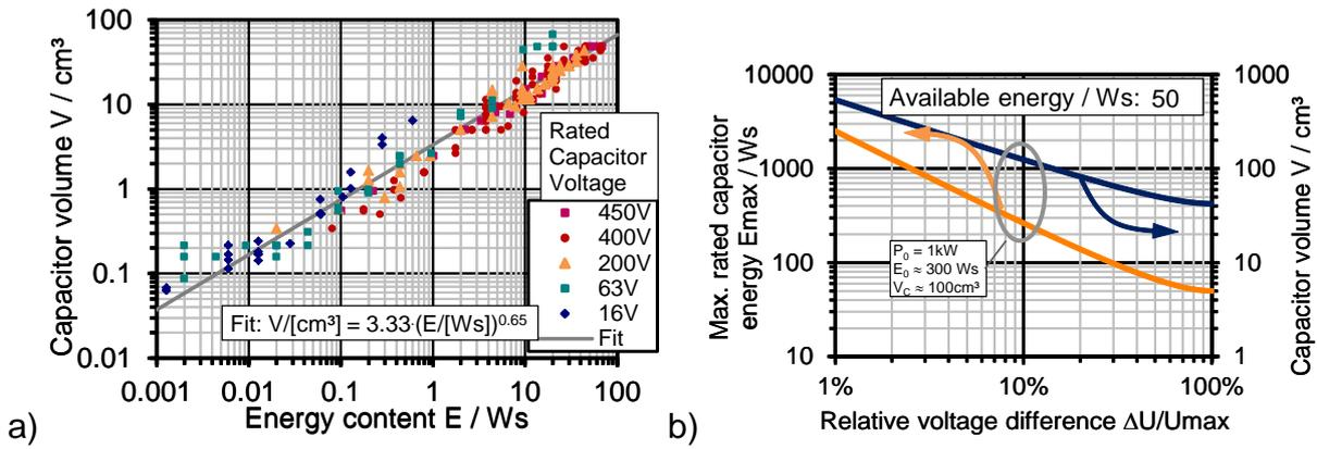
Figure 1: Volume size of electrolytic capacitors. a) Various electrolytic capacitors, data from [5]. b) Needed capacitor energy and volume size to store 50 Ws.
