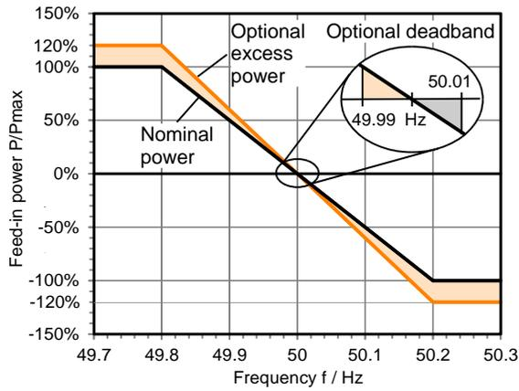
Figure 5: Degrees of freedom of the power delivery curve. According to [12].
