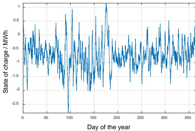
Figure 6: Calculated battery state of charge with frequency compensation using only a running average with an averaging length of one day for a battery storage with 1 MW rated Primary Control Power.
