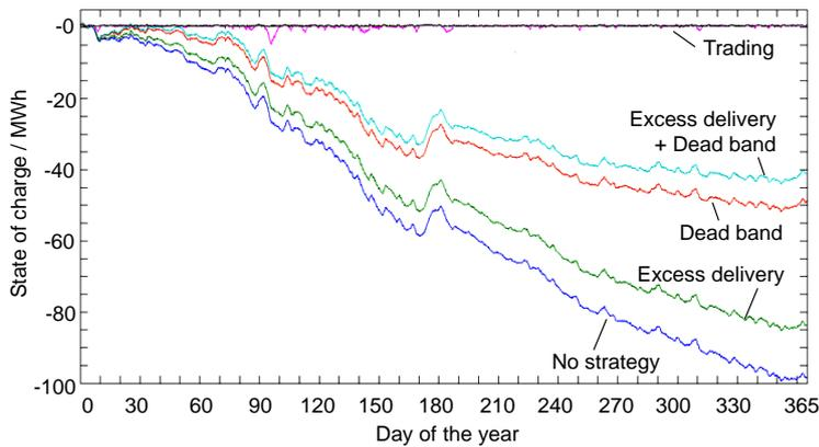
Figure 4: Effect of applying degrees of freedom for a battery storage with 1 MW rated Primary Control Power [14].
